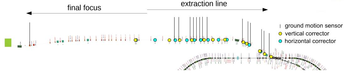
• 22 dipole corrector magnets in extraction line
