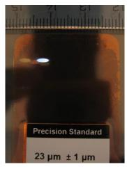
FDSCI setup calibrated by comparing the optical thickness of five individual calibration samples to the certified geometric thickness.
