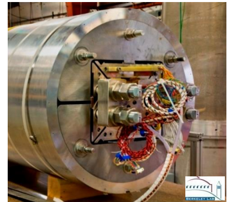
HD2: highest bore field in accelerator dipole (13.8 T)
