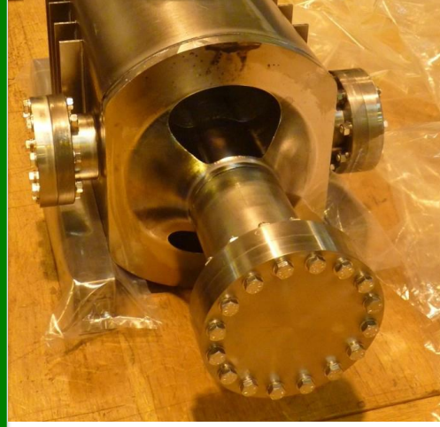
4-rod in SM18 for RF measurements [Lancaster UK]
