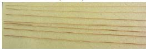
25 cm Anthracene Core Quartz Capillary Fibers
