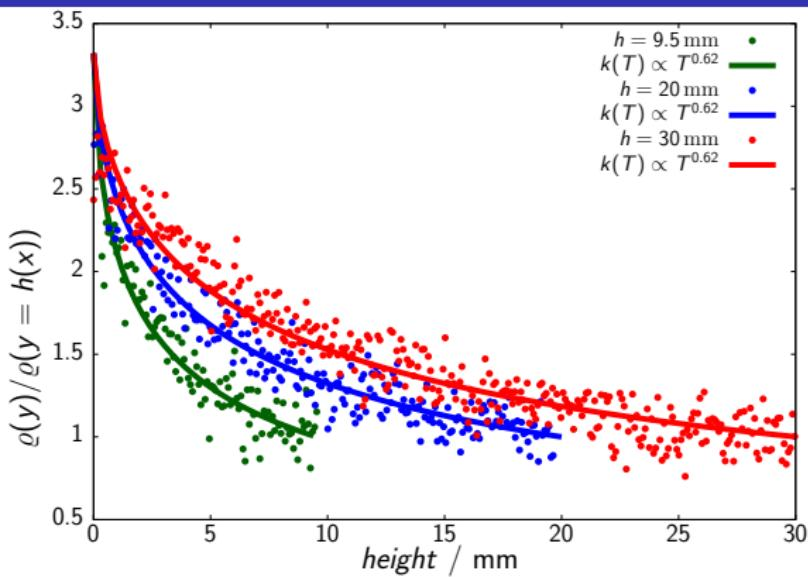
Wedge shaped cell:  $T_{high} = 26.1$  K,  $T_{low} = 7.86$  K and  ${}^3\text{He}$  pressure 9 mbar.
