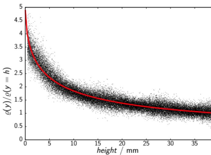
Measured gas density gradient for the rectangular shaped cell.
