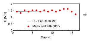
Sufficiently homogeneous resistance between copper electrodes
