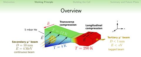
The compression process can be decomposed into three stages:
