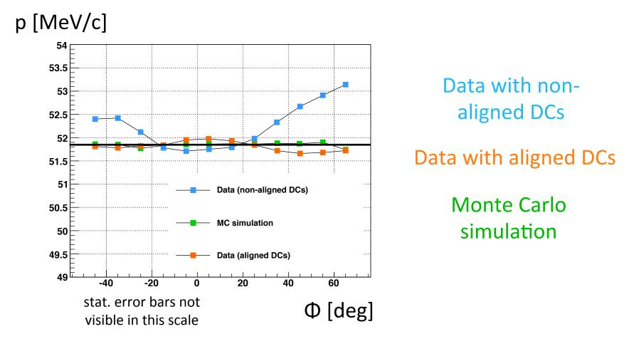
Comparison Mott line for non- and aligned DCs
