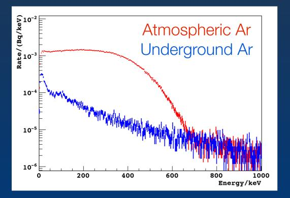
Identified source of underground argon in Colorado measured to have <<u>6.5mBq/kg</u> i.e. > 150 times lower rate compared to atmospheric argon Plant (including cryogenic distillation at FNAL) produces ~0.5 kg/d
