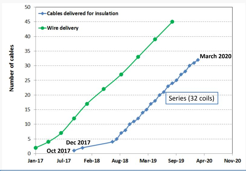
**Delivered** to magnet team: 2 months before coils assembly (for electrical insulation) **Available**: availability of cables according to wire delivery schedule
