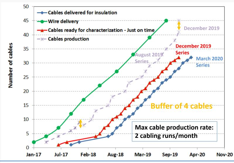
**Delivered** to magnet team: 2 months before coils assembly (for electrical insulation) **Cables ready for characterization** : <u>3 months</u> before delivery to magnet team **Available**: availability of cables according to wire delivery schedule
