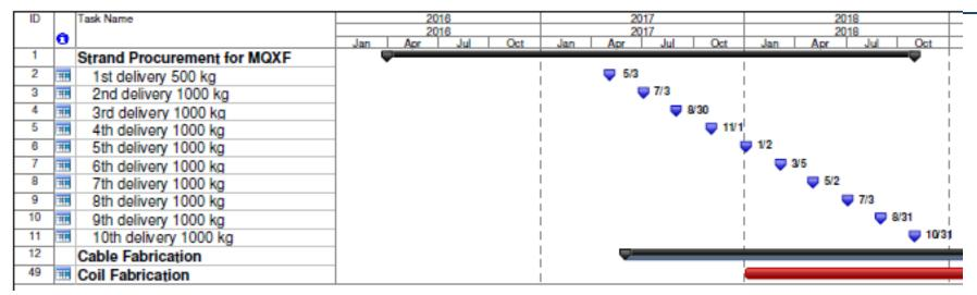
OST (most likely vendor for RRP wire) has sufficient capacity to handle both CERN and US orders in the same time frame. Production rate ~ 1 metric ton/month. During ITER the production rate was ~ 2 tons/month.
