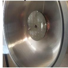
Laser power meter measures power delivered through ion source readout via existing thermocouple infrastructure
