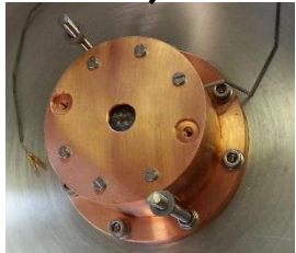
Laser power meter measures power delivered through ion source readout via existing thermocouple infrastructure
