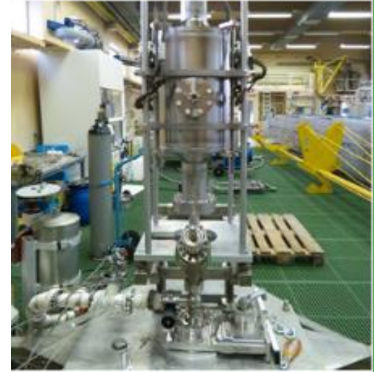
4-rod prepared for rinsing @ CERN
