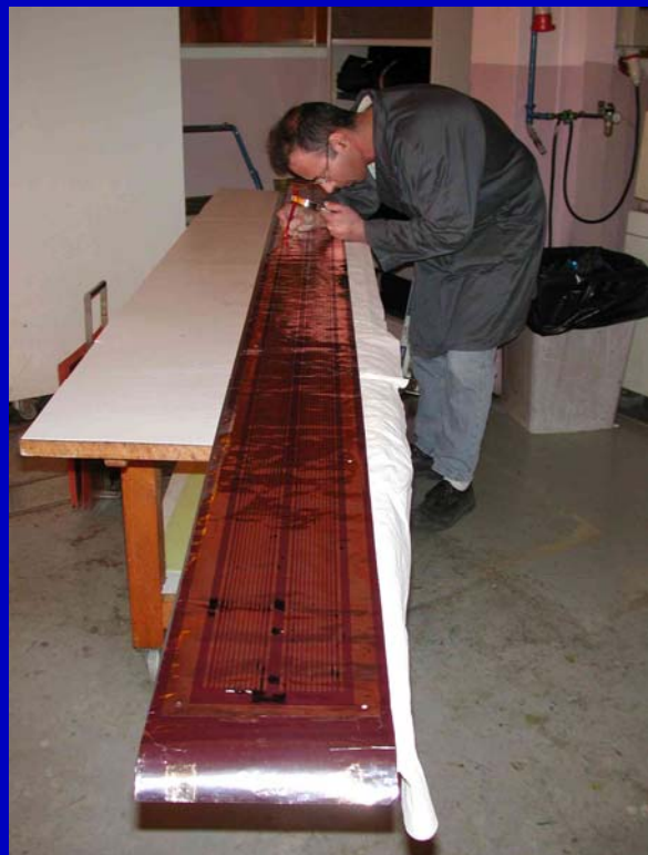
4 meter long flex LHC injection kicker prototype
