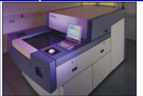
Figure 2 e 3 – The Paragon-8000 Laser Direct Imaging system (above) and 25 µm features exposed using this system (below)
