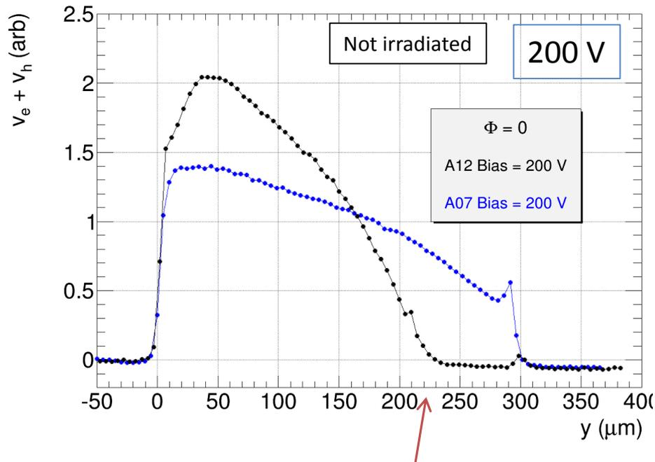
→ expected depletion depth for A12A at 200 V 220  $\mu\text{m}$ !
