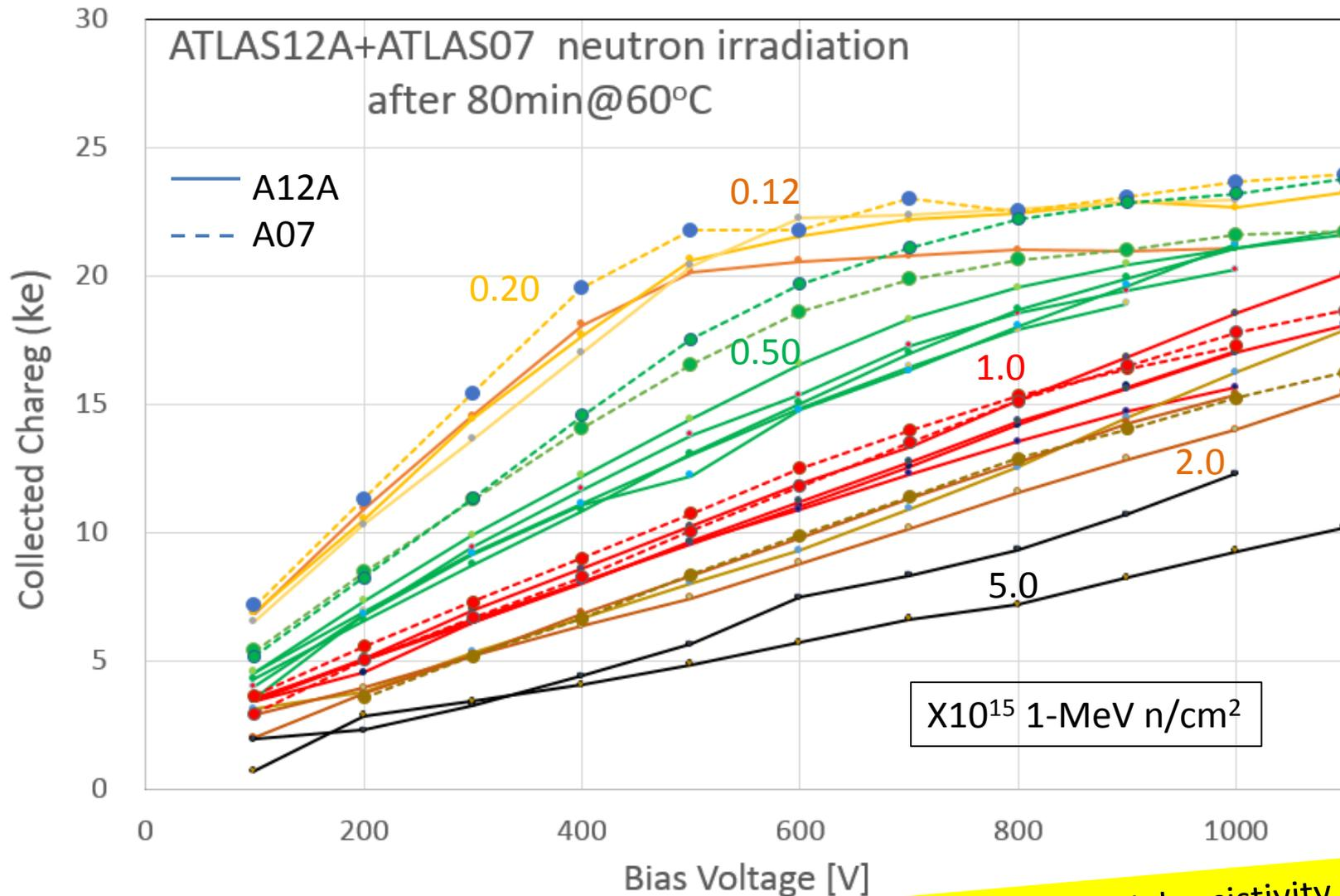
Consistent curves: A07 yields larger at low fluence and low bias: different initial resistivity
