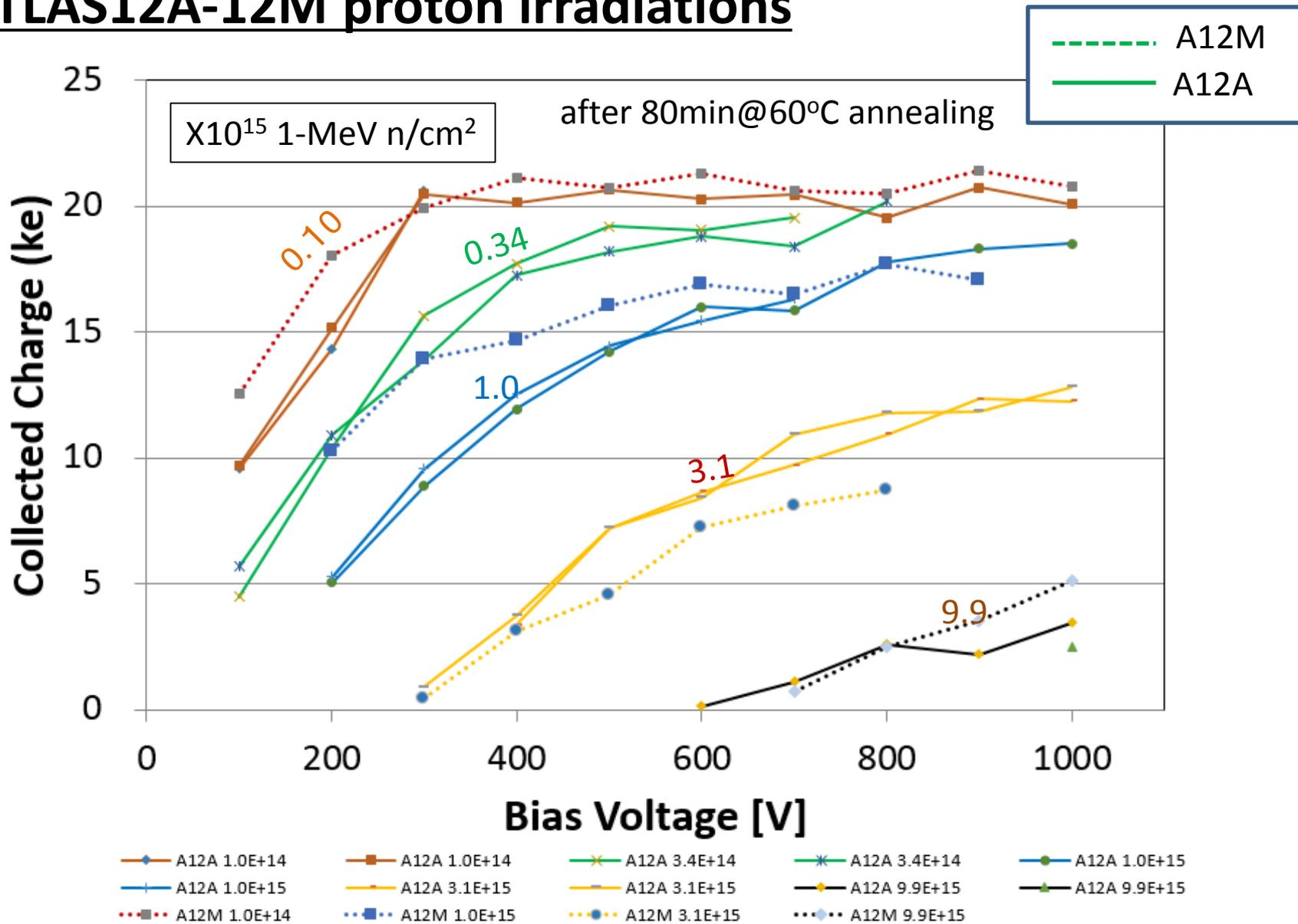
12M yields larger signal at low fluence and at low bias: different initial resistivity
