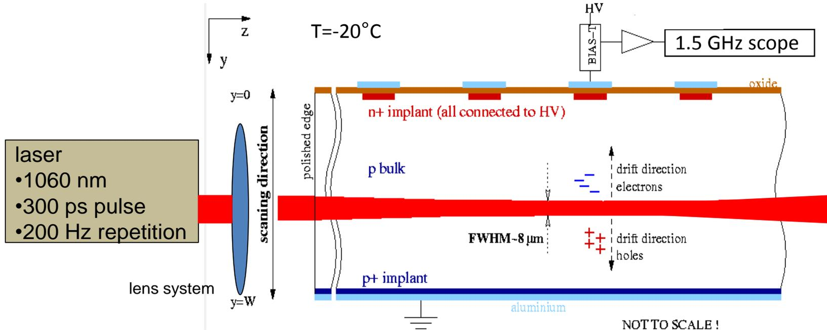
IR laser injected from polished side
