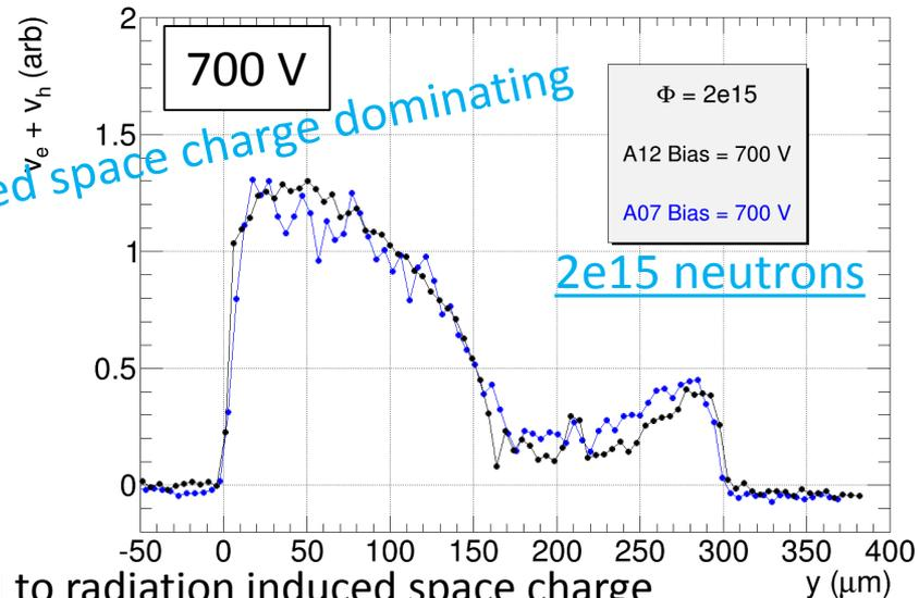
→ contribution of initial space charge small compared to radiation induced space charge
