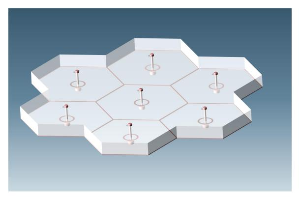
In this illustration, the viewer is looking down through dielectric (transparent here for clarity). A small copper button is the only metallic electrode presented to the charge arriving from the drift region. The grid has been placed on the underside and a small circular guard ring has been added to capture surface currents that would, if allowed to reach the electrode, increase noise.
