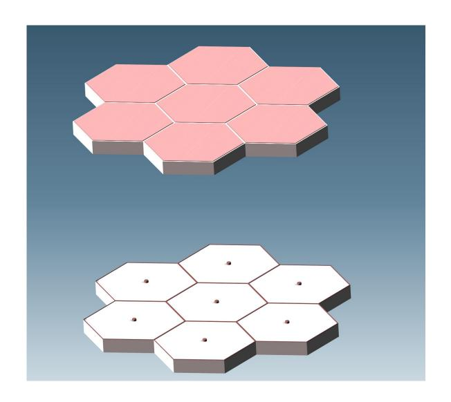
Two pixel plane designs. The top has simple copper pads connected by vias to the circuits behind. The size of each pixel is about 3 x 3 mm<sup>2</sup>
