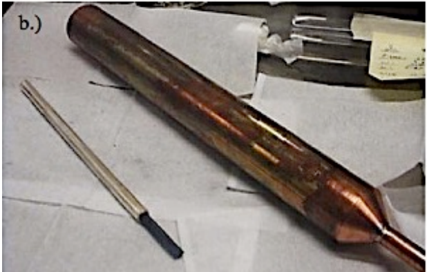
bar assembled in a Ag monocoresh billet.
