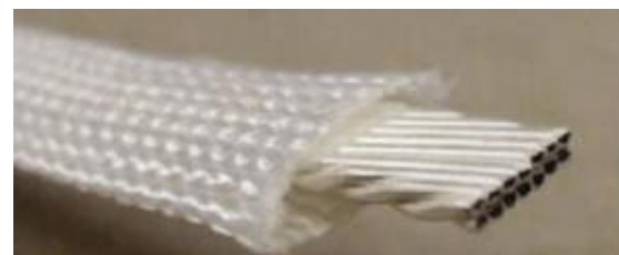
Rutherford cable by LBNL
