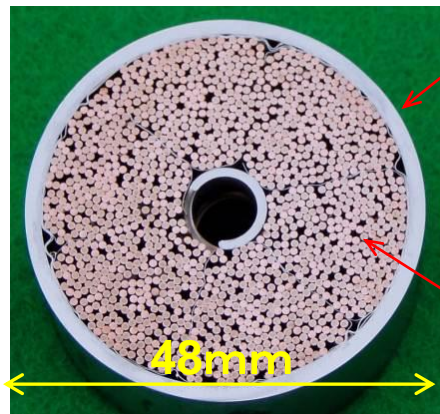
ITER/TF Nb 3 Sn wire ( 0.82mm dia. with Cr plating)
