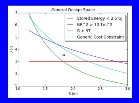
Under these assumptions, detector must live in this region (\*). Cost increases more quickly with R than B. Exact behavior is detector technology dependent. Guess B<sup>1.5</sup> (R+1)<sup>3</sup>
