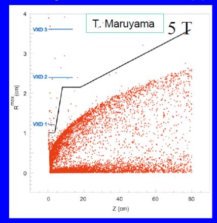
Inner radius of vertex detector scales as 1/√B. Important for MS term of IP resolution.
