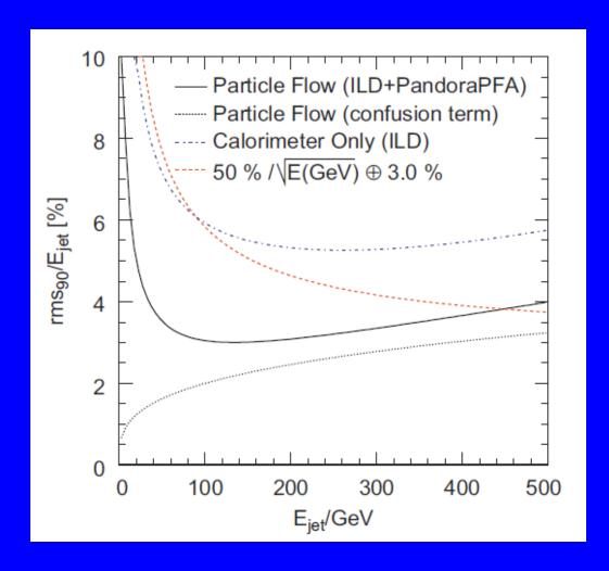
ILD design works well across the full ILC jet energy range (45 GeV to 500 GeV).
