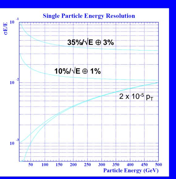
ECAL and HCAL based energy measurements for charged particles are not competitive with design momentum resolution over the complete ILC envisaged energy range.
