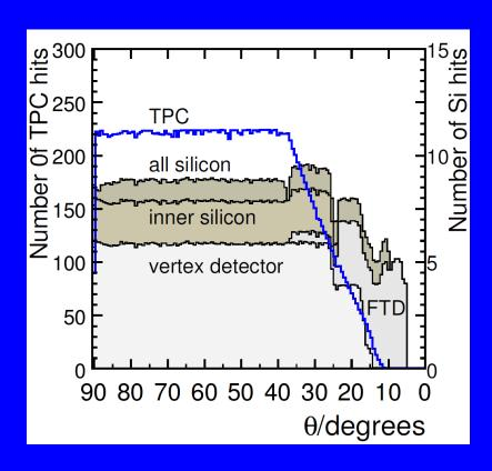
Complete TPC coverage to  $37^{\circ}$  VTX + SIT + FTD + SET + ETD => precision, redundancy and coverage to  $|\cos\theta| = 0.996$ .
