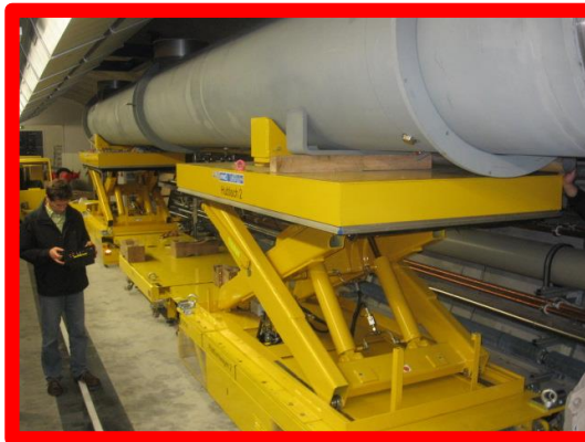
DESY XFEL installation Capacity: 6.t per lifting platform Lifting height: 2.4m
