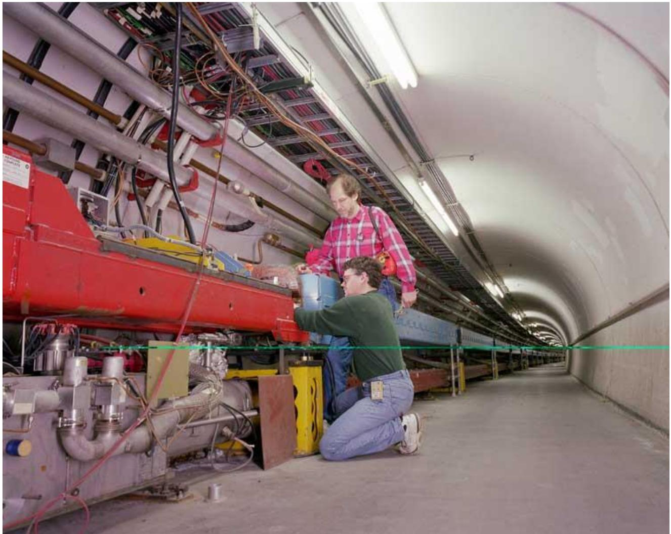
Fermilab's superconducting Tevatron can just be seen below the red and blue room temperature magnets of the 400 GeV main ring.
