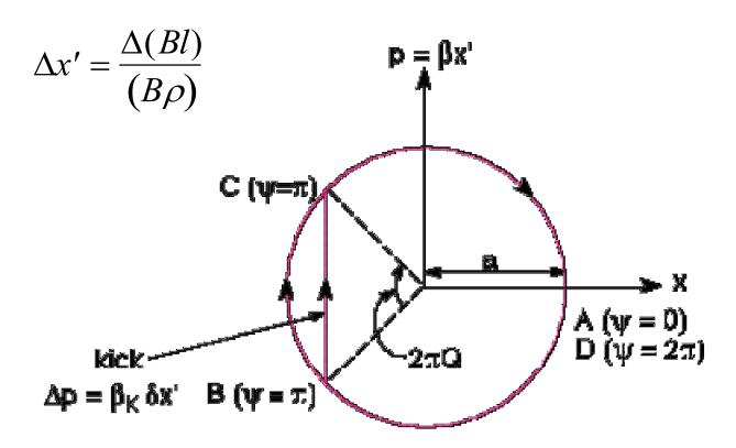
Tracing a closed orbit for one turn in the circle diagram with a single kick. The path is ABCD.
