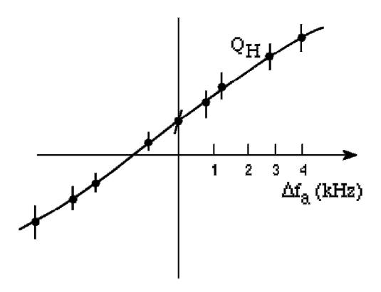
We can steer the beam to a different mean radius and a different momntum by changing the rf frequency and measure Q
