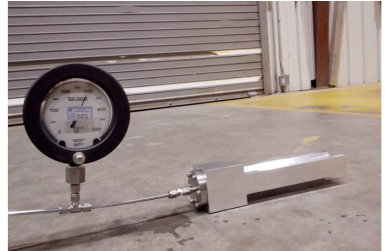
Test cell factor ~10 safety test, burst pressure above 3500 psi
