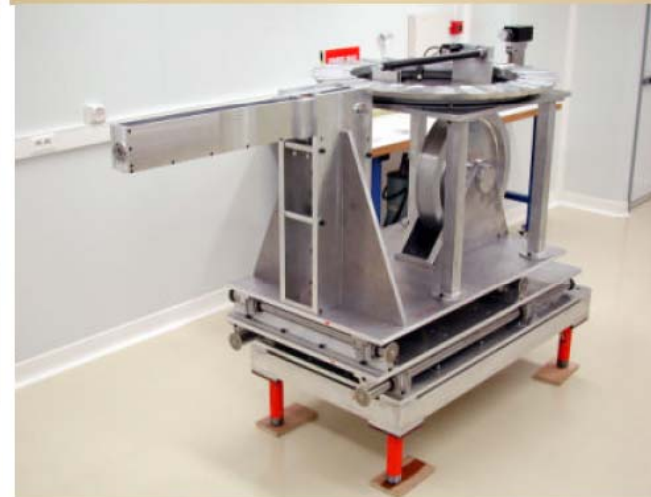
"Carousel" brick dispensing and storage system
