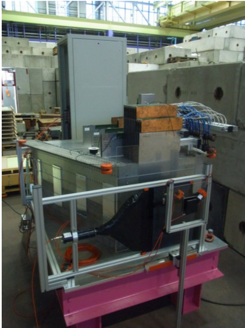
“ILD like” absorber structure with up to 14 layers of different size
