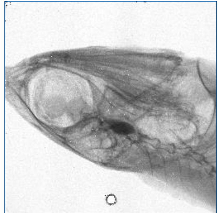
First image obtained with a TSV processed hybrid pixel detector (flat field corrected)
