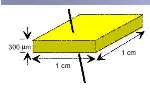
Intrinsic silicon will have electron density = hole density; 1.45 10<sup>10</sup> cm<sup>-3</sup> (from basic semiconductor theory).
