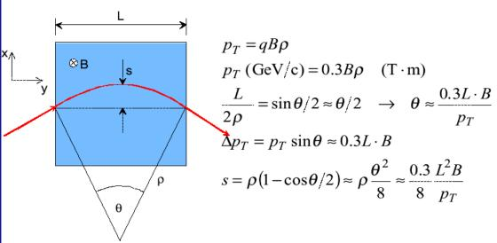
the sagitta s is determined by 3 measurements with
