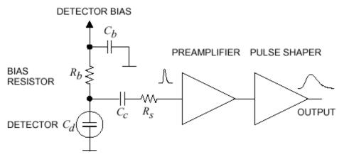
where the detector is represented by the capasitance  $C_d$ , bias voltage is applied through  $R_b$ , and the signal is coupled to the amplifier though a capasitance  $C_c$ . The resistance  $R_s$  represent all the resistances in the input path. The preamplifier provides gain and feed a shaper which takes care of the frequency response and limits the duration of the signal.
