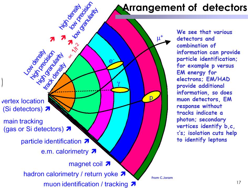
information can provide particle identification; for example p versus EM energy for electrons; EM/HAD provide additional information, so does muon detectors, EM response without tracks indicate a photon; secondary vertices identify b,c,  $\tau$ 's; isolation cuts help to identify leptons
