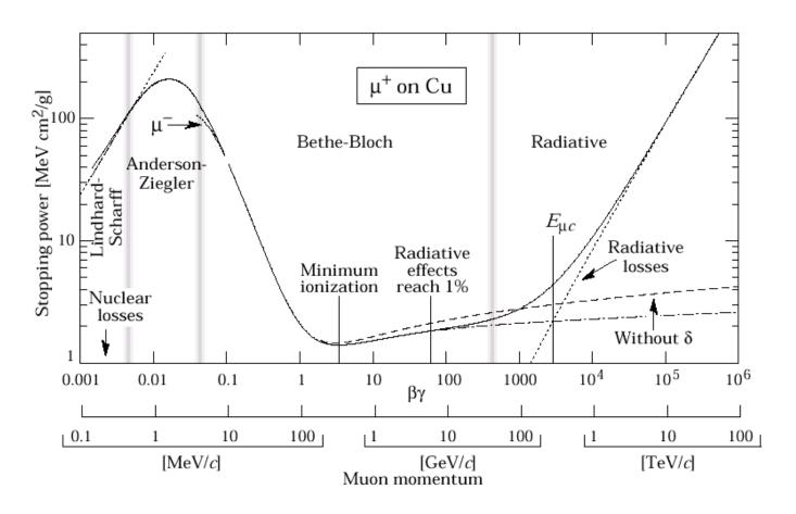
$$\left\langle \frac{dE}{dx} \right\rangle = -4\pi N_A r_e^2 m_e c^2 z^2 \frac{Z}{A} \frac{1}{\beta^2} \left[ \frac{1}{2} \ln \frac{2m_e c^2 \gamma^2 \beta^2}{I^2} T^{\text{max}} - \beta^2 - \frac{\delta}{2} \right]$$
