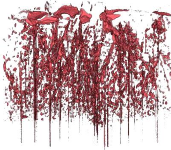
Pore reconstruction in a section (pixel size) of Nb coating
