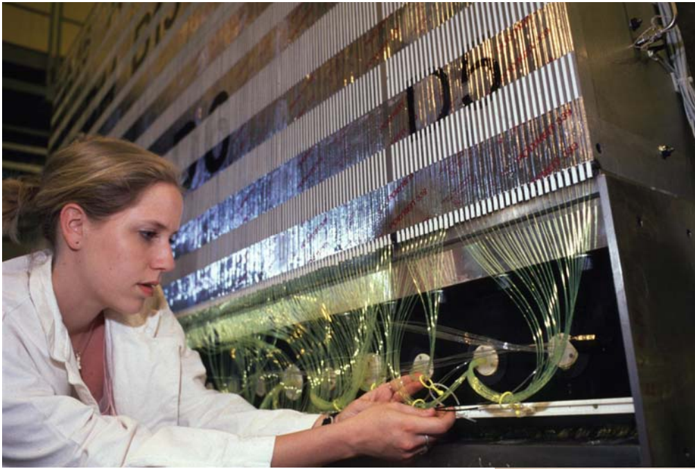
Wavelength-shifting readout fibres grouped to define the pointing cell structure
