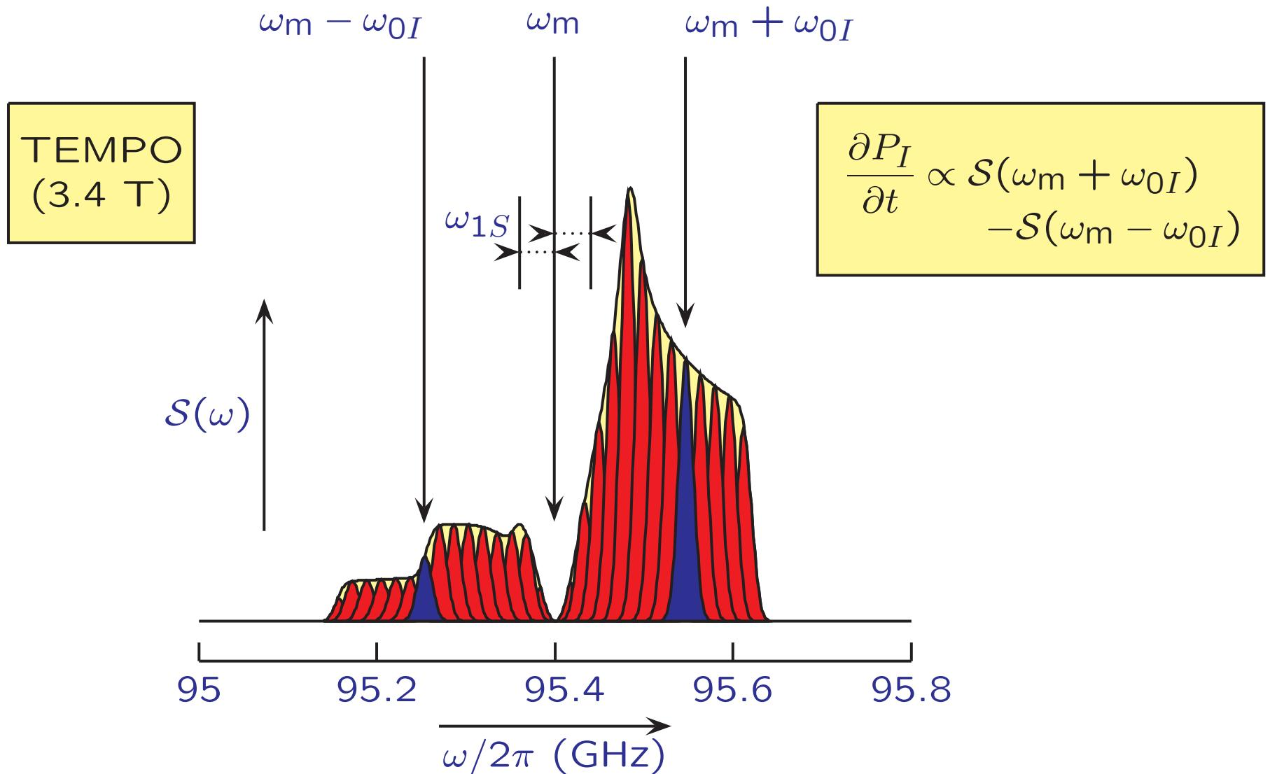
strong  $\mu$ -wave field:  $\omega_{1S}T_{2S} > 1$   $\longrightarrow$  differential solid effect
