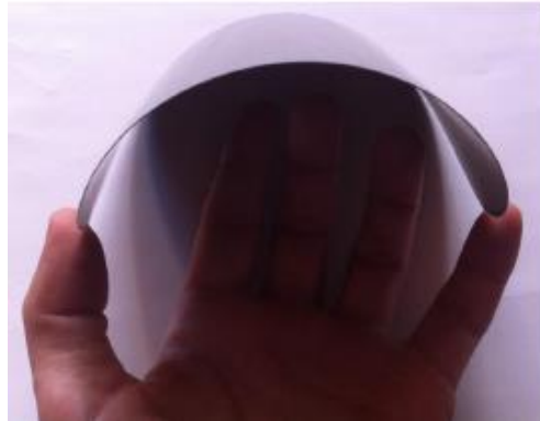
Wafer thinned to 50 \mu\text{m}
