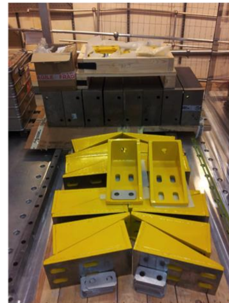
Underfloor columns, brackets & ties
