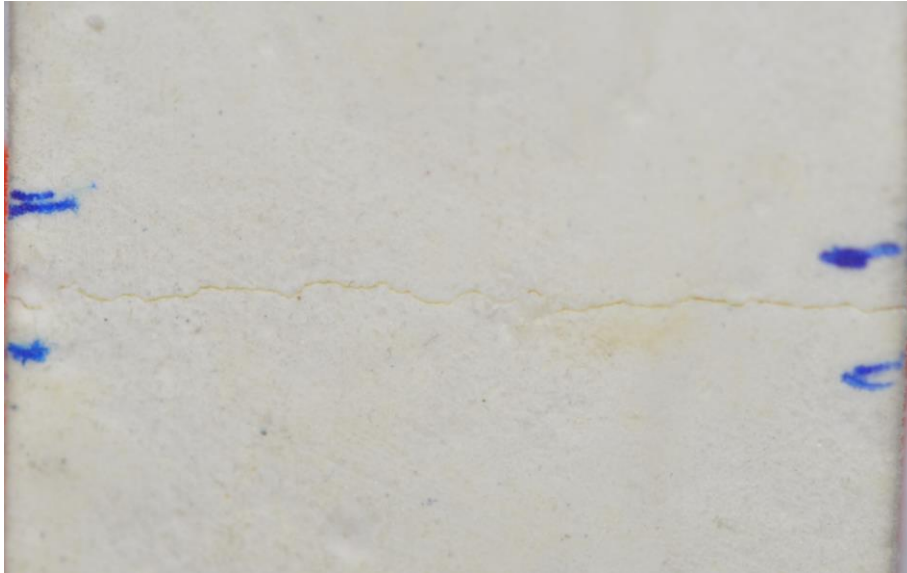
Crack while actively cooling
