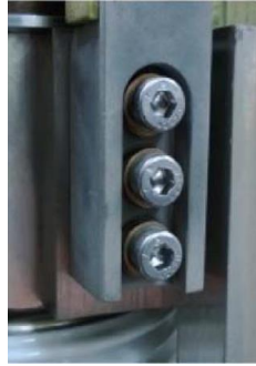
3-screw bolted contact on quadrupole diode stacks
