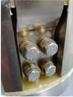
4-screw bolted contact on dipole diode stacks
