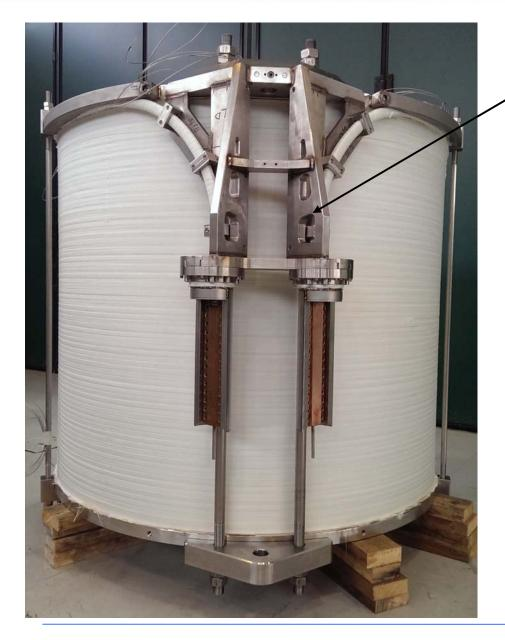
Stainless steel structure providing mechanical support to terminations
