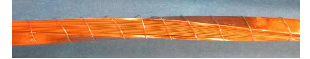
This work characterizes the electromechanical behavior of two commercially available REBCO tapes (SuperPower and SuNAM) under tension and combined tension-torsion using structural finite element analysis (FEA) and experimentation at 77 K and in self-field conditions.
