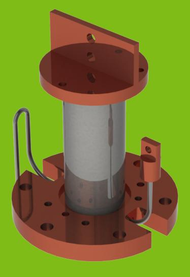
A gas gap heat switch was designed, built, assembled and tested at 4 K upon the requirements established as per IUAC cryogen-free magnet The good agreement between the calculated and measured values enables a useful extrapolation for several and new applications, such as the one described in this document, where a completely cryogen-free
