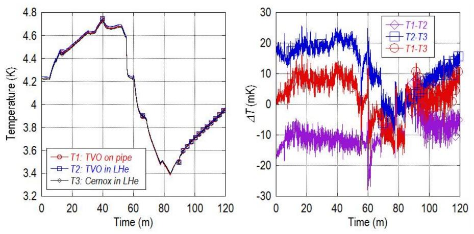
Any differences between two sensors are less than 30 mK
