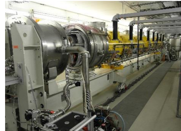
■ XATB – module inside radiation protection shielding
