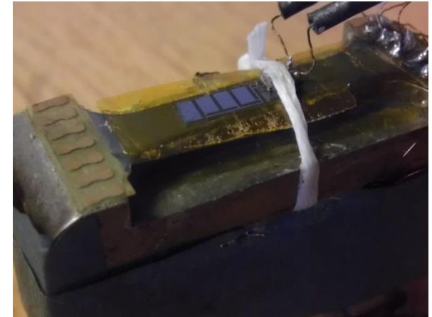
U-spring with etched thin film
