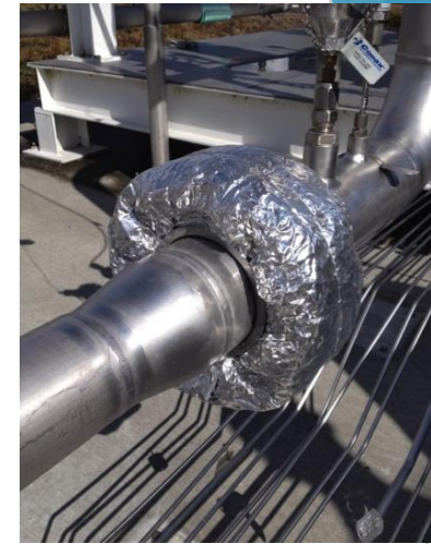
LCX on a simulated vehicle tank (left) and piping flange assembly (right) on the SPLS
