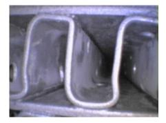
• Cold box and HX manufacturer, as well as, JLab did not believe this was related to the high LN usage unless this was residual from moisture (which caused blockage of some of the passes)
