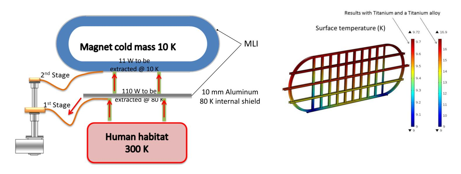
Multiple simulations have been performed to evaluate the heat fluxes reaching the surface of the magnet depending on its temperature :
