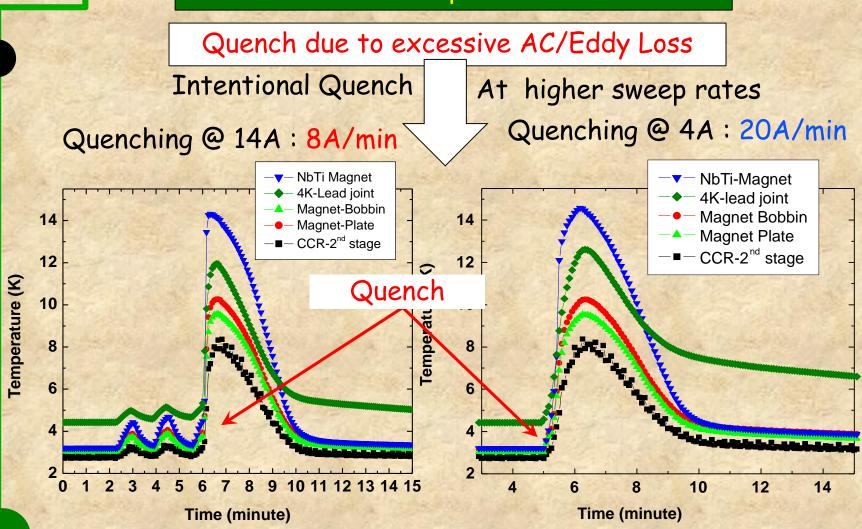
Dynamic Losses @ 8A/min at 14A~ Losses @ 20A/min at 4A
