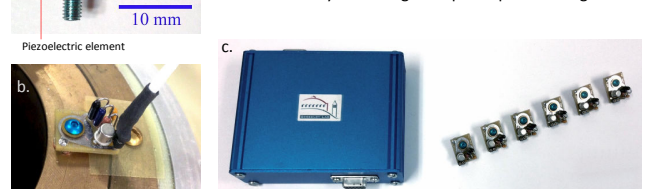
Fig. 4. (a) Acoustic emission sensor (side view). (b) Sensor installed at the end of a CCT magnet (two sensors at the opposite ends were installed) (c) Components of a six-sensor acoustic quench localization system built for future studies.
