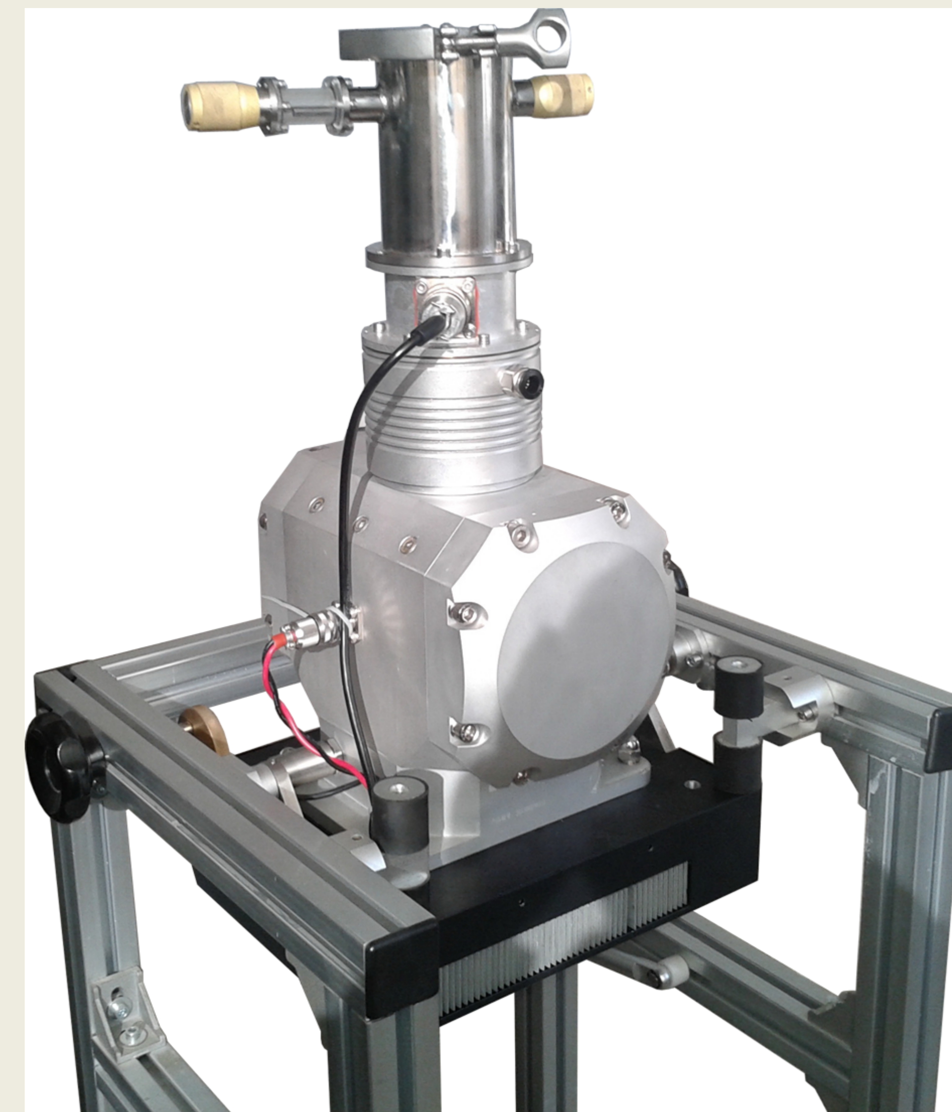
Figure 5. Photo of the developed cryogenic tensile testing apparatus.
