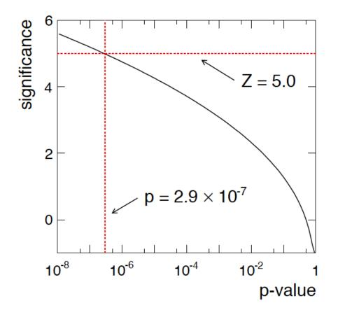
In fact this tradition should be revisited: *p*-value intended to quantify probability of a signallike fluctuation assuming background only; not intended to cover, e.g., hidden systematics, plausibility signal model, compatibility of data with signal, "look-elsewhere effect" (~multiple testing), etc.
