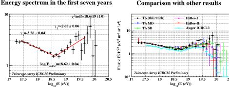
21% systematic uncertainty on energy scale; fluorescence (11%), atmosphere (11%), calibration (10%), geometry (4%) and reconstruction (10%).
