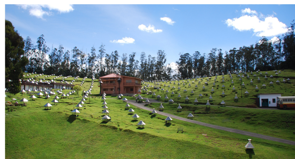
Figure 1 : View of the GRAPES-3 experimental site at Ooty with the scintillator detector array, control room building (center) and muon detector buildings (left).
